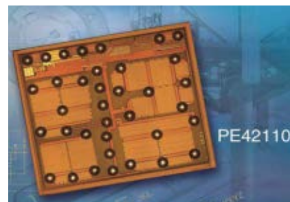
▲ Fig. 8 SP9T CMOS switch (courtesy of Peregrine Semiconductors).
