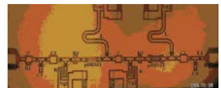
▲ Fig. 5 The two-stage PA chip.
